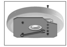
Secure the antenna to the mount base using bolts, spring washers, and flat washers.
